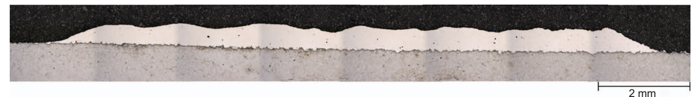
Figure 5 Wide Stellite-6 coating on steel.
