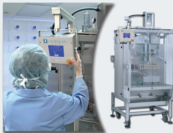
FIGURE 1 | The Hydropac AWS-5000 Pouch Machine automatically forms, fills, and seals pouches using a continuous roll of special plastic film stock. A touch screen panel located on an articulating arm activates all control functions.
