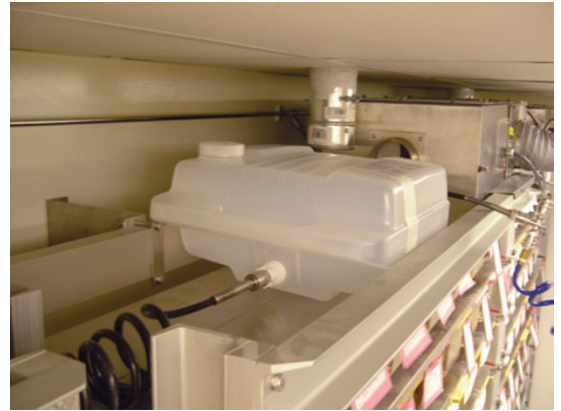
FIGURE 3 | A carboy on a ventilated rack for delivery of ivermectin-treated water through the automatic watering system.
