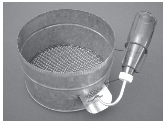
FIGURE 1 | The cage has grids at the bottom so that animal excreta can pass directly through the bottom. The spill canal collects any water that animals spill and facilitates measurement of the actual water intake.
