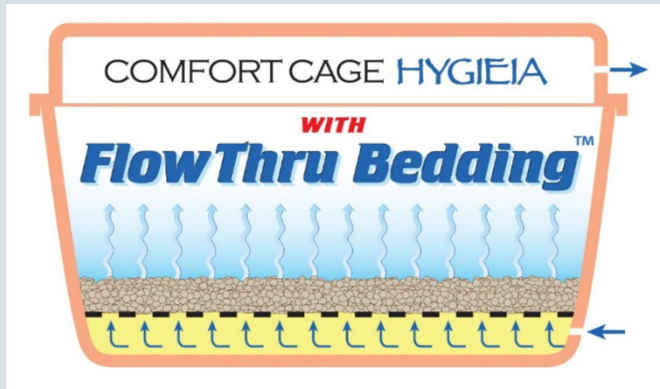
FIGURE 2 | The Flow Thru Bedding design allows fewer ACH to keep the bedding dry and reduce the atmospheric ammonia content as compared to standard IVC designs.
