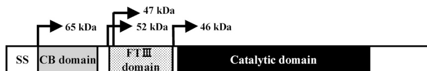
Fig. 7 Schematic representation of chitinases encoded by chi65 .
