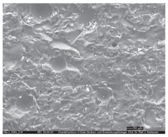
Figure 6 SEM image of representative sample of porcelain ground with the coarse diamond instrument. Original magnification ×500. The surface reveals a maze of steep ridges, grooves and voids. SEM, scanning electron microscopy.
