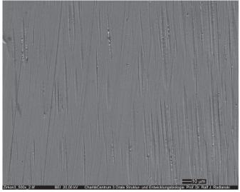
Figure 3 SEM image of zirconia sample ground with the coarse diamond instrument. Original magnification ×500. SEM, scanning electron microscopy.
