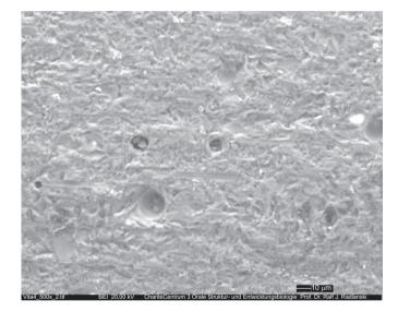
Figure 7 SEM image of porcelain sample ground with the three diamond instruments and then polished using the coarse polisher. Original magnification  $\times$ 500. SEM, scanning electron microscopy.
