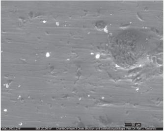
Figure 8 SEM image of porcelain sample ground with the three diamond instruments and then polished with the three polishers. Original magnification ×500. SEM, scanning electron microscopy.
