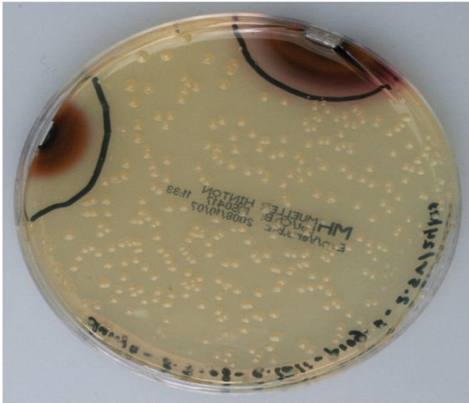
Figure 3 Discoloration of MHA medium observed at anodes when bacteria ( E. coli ) were exposed to 27 \text{ V}\cdot\text{m}^{-1} . MHA, Mueller-Hinton agar.
