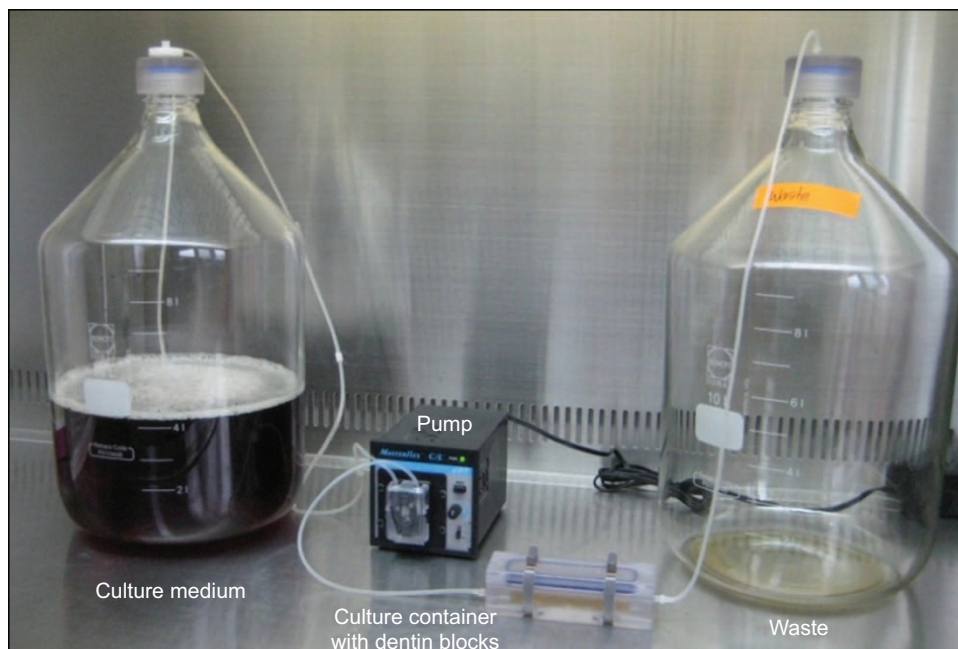
Figure 1 Luppens apparatus. The apparatus consisted of a vessel containing media, a pump, a culture container and a vessel with waste, all connected by silicone tubing.
