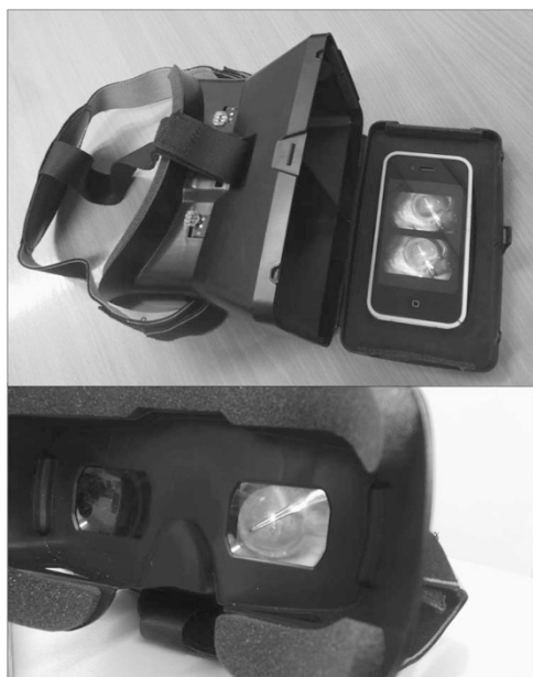
Figure 2 iPhone loaded into the VR headset for viewing of video with stereoscopic 3D effect.
