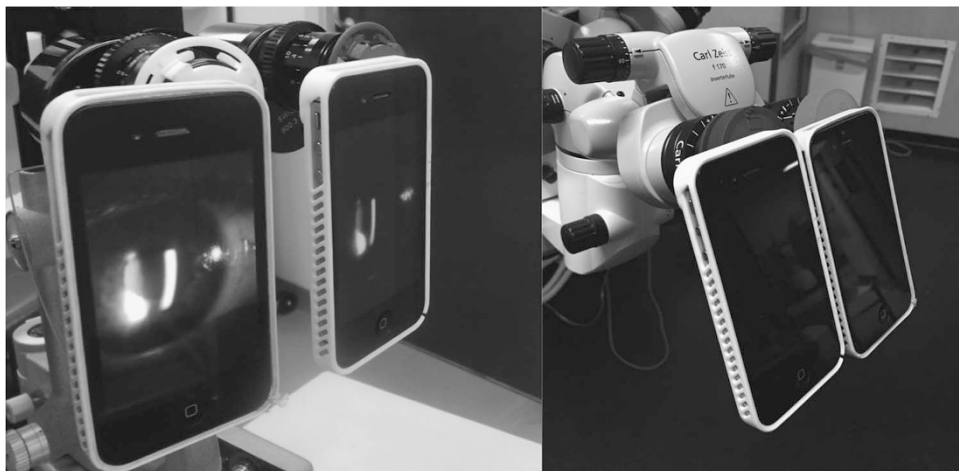
Figure 1 Two phones attached to the slit lamp or microscope eyepieces record images from two perspectives to create a stereoscopic effect.
