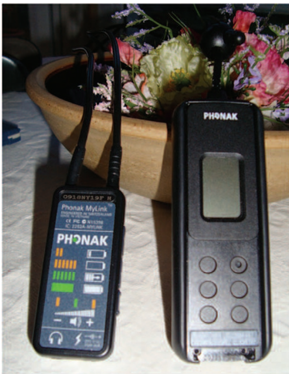
Figure 2 Patient's transmitter and receiver devices. The transmitter is on the right (ZoomLink+, Phonak, Switzerland) and is placed on the surgeon's person. The receiver on the left (MyLink+, Phonak, Switzerland) is held by the patient. The receiver is set to pick up auditory signals from the transmitter, which is in turn picked up by the patient's hearing aid.
