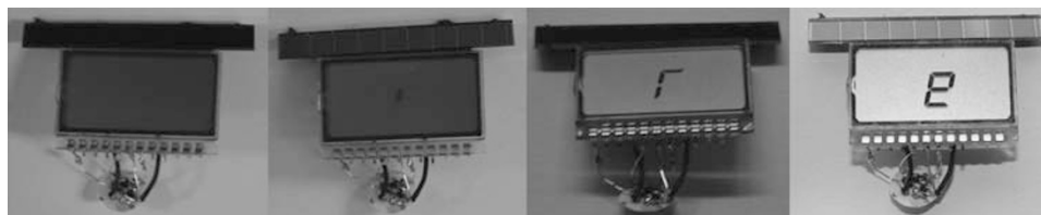
Figure 7 Demonstration of the passive circuit, showing increasing ambient light from left to right. The different activated segments represent the decreasing pupil size using this entirely self-powered scheme.
