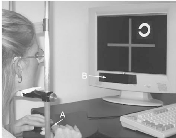
Figure 1 Testing apparatus: Patient in chin rest is tested monocularly with appropriate correction and add for screen distance. The patient signals their response to orientation of a tumbled Landolt C that is flashed on screen by pressing one of the four buttons on the button pad (A). Fixation is monitored with an infrared pupil and corneal reflex camera (B) mounted in box on the bezel of monitor. The testing is conducted in a room darkened to <1 \text{ Cd/M}^2 .
