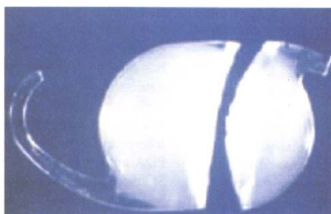
Fig. 2. Gross photograph of one of the explanted single-piece SC60B-OUV lenses, manufactured by MDR, Inc., Clearwater, FL, USA. This opacified IOL was explanted after bisection and submitted to our laboratory by Dr Nitin Anand of Luton, UK. Note the opacity of the central optic area and a clear band approximately 1 mm wide subtending the optic. The IOL's haptics are also clear.
