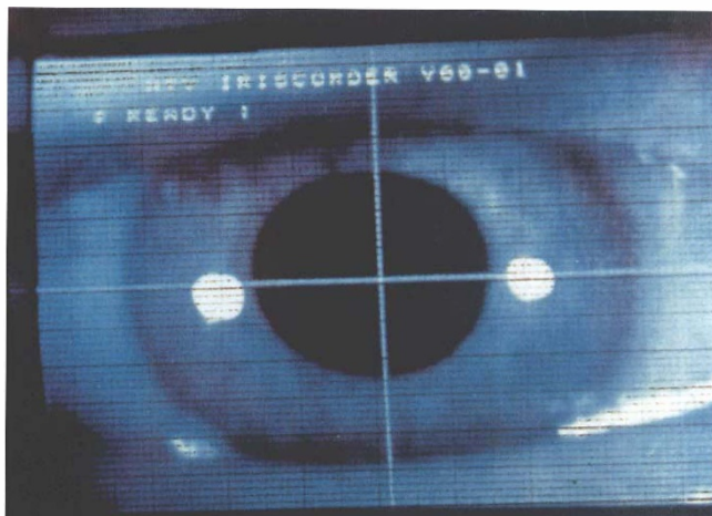
Fig. 2. Hamamatsu C301 Iriscorder videopupillograph television system for pupil image viewing.
