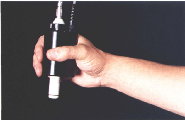
Fig. 1. Motorised transducer holder. The white ultrasound transducer has been coupled with the black motorised holder.
