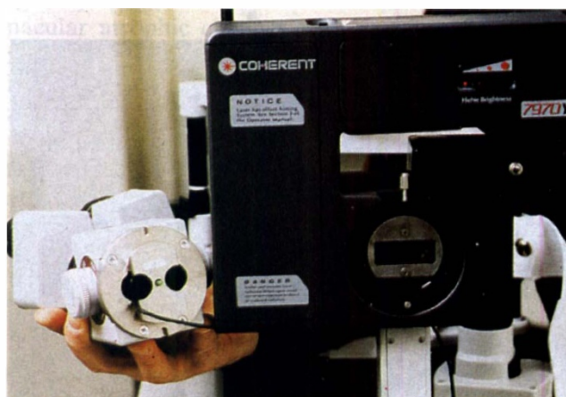
Fig. 2. The microscope optics come away from the main laser body by loosening a screw. The fixation light is fitted in the microscope mounting plate between the objective lenses.
