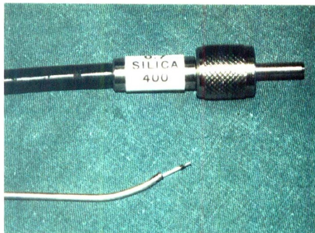
Fig. 3. A 400 mm plain optical fibre in the angled holder. Note the charring of the outer plastic sheath and the 3 mm of bare fibre at the tip.
