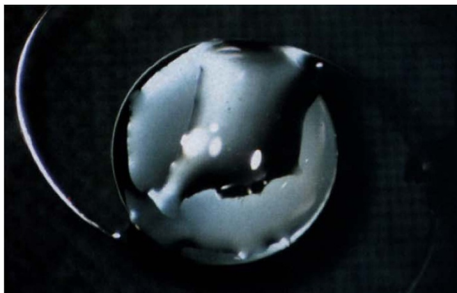
Fig. 3. Heparin-coated polymethylmethacrylate (PMMA) IOL after incubation with neat silicone oil. Irrigation failed to remove the oil from the IOL surface.
