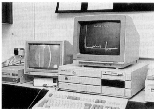
Fig. 1. The Oxford Modular Cataract Image Analysis System.
