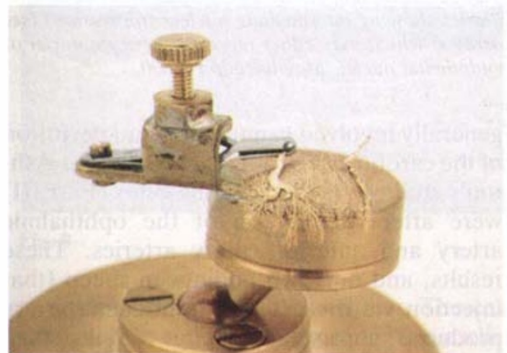
Fig. 4 Choroid fragment held by bulldog on dissecting stand with two ball and socket joints allowing large range of movement for orientation of specimen under dissecting microscope.
