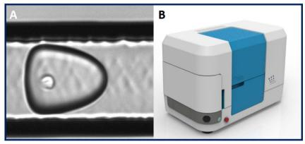
Figure 1: Cyto-Mine is the first integrated device to rapidly and automatically measure secreted protein from individual cells to identify rare and valuable variants. (a) A picodroplet containing a single cell prior to being dispensed into a single well of a microtiter plate. (b) The Cyto-Mine Single Cell Analysis and Monoclonality Assurance System.
