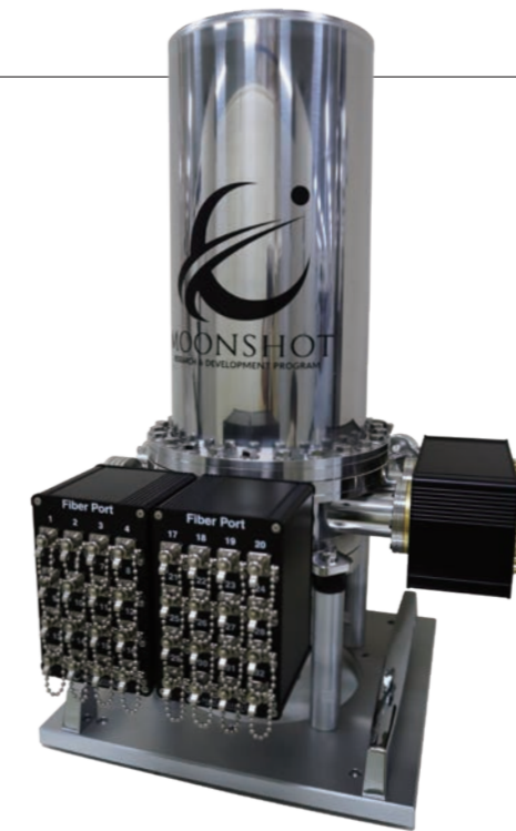
▲ In a project led by Takashi Yamamoto of Osaka University, a team at the company Hamamatsu Photonics is developing a large-scale detector system that uses superconducting nanowires to measure single photons.
