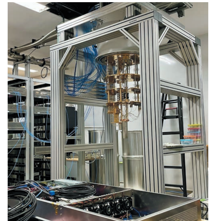
▲ A quantum computer at Osaka University based on superconducting qubits developed by RIKEN and using a controller made by QuEL and others.
