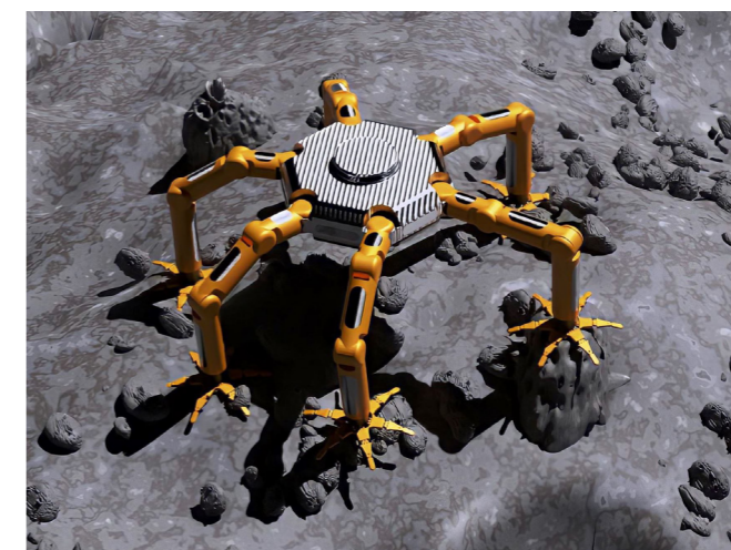
▲ A simulation of Hayabusa touching down on the asteroid Itokawa (top); Space Capable Asteroid Robotic Explorer (SCAR-E), a crab-like, six-legged robot that can grip and walk across surface of an asteroid (bottom).
