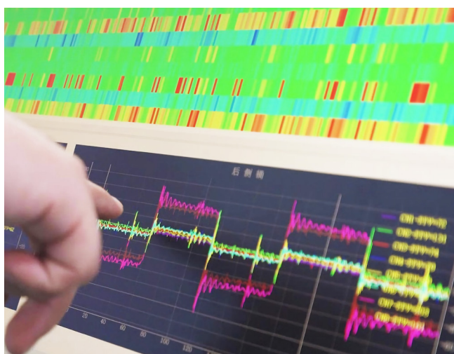
▲ The signal patterns of ultrasonic sound waves can be analysed for internal changes in lithium-ion battery cells.
