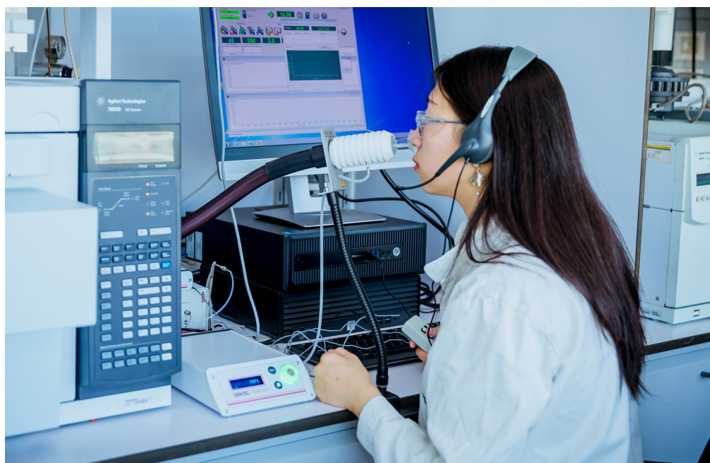
Figure 2. A researcher uses an instrument called a gas chromatograph (GC). The process of gas chromatography-olfactometry (GC-O) uses a GC to separate the volatile compounds, and then the odour is detected using an olfactometer.
