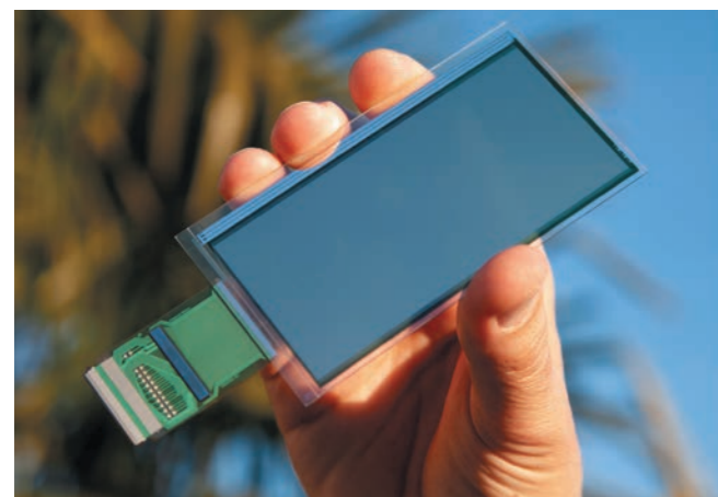
▲ A photodetector based on fullerenes (left) could be integrated in smartphones and enhance their security by turning the whole screen into a fingerprint reader. The curved surface of a wind-turbine pole (right) is covered with solar cells that incorporate fullerenes.
