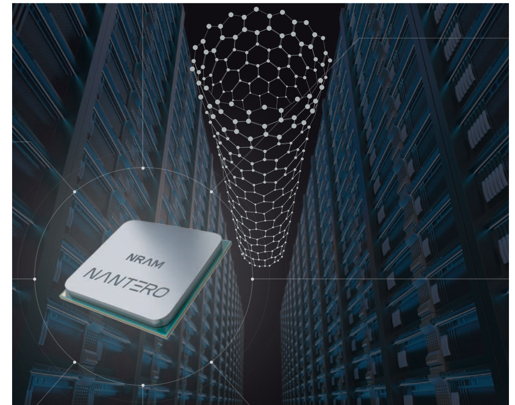
▲ Low-power, non-volatile nano-random access memory (NRAM) based on carbon nanotubes could drastically reduce the power consumption of data centres.
