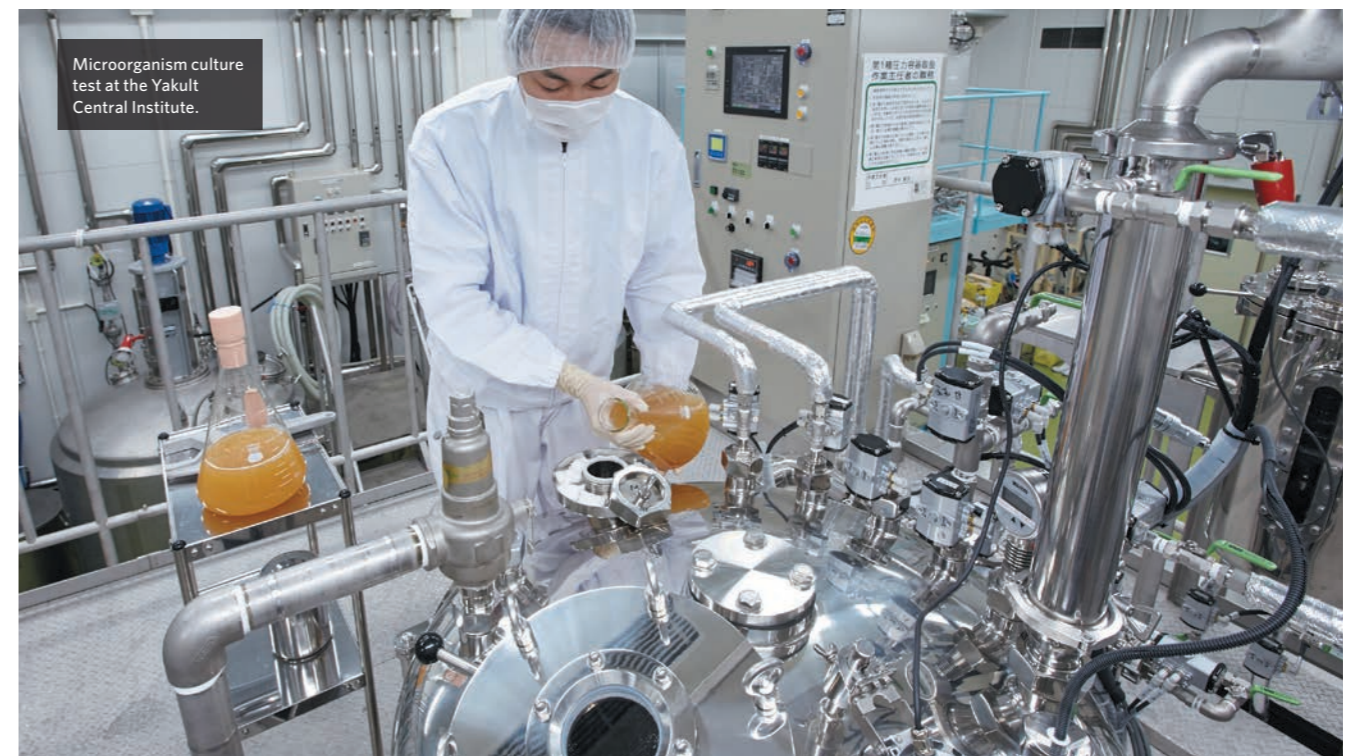
Jar fermenters at microbial culture testing stations at the Yakult Central Institute.
