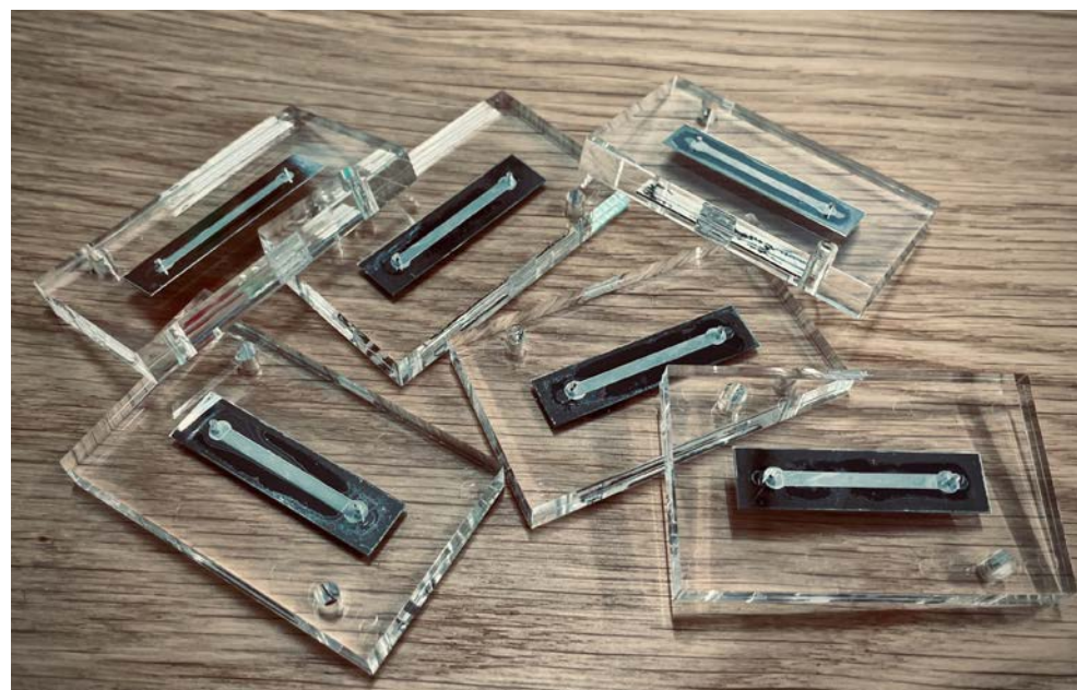
A device developed by Craif consisting of zinc oxide nanowires embedded in a microfluidic channel is designed to more effectively extract exosomes from urine.
