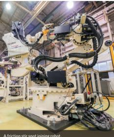
A friction stir spot joining robot
