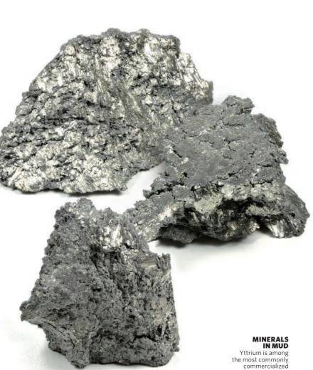
Yttrium is among the most commonly commercialized rare-earth elements, used to produce phosphors for cell phones, display screens and LEDs. Promotion Program, to come up with high-efficiency, low-cost deep-ocean resource surveying and extraction systems. New deep-water acoustic mapping technologies, exploratory autonomous vehicles and mud pumping machinery are in early testing.
