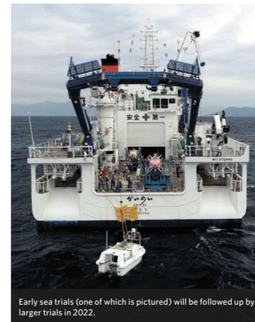
In 2019, a prototype underwater acoustic communication system was mounted on a number of AUVs and an autonomous surface vehicle for testing.
