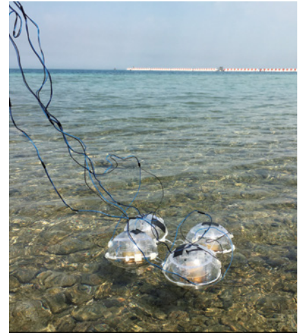
A field test for the spherical spring-assisted triboelectric nanogenerator is performed in the sea.
