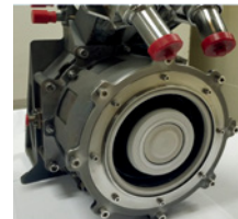
Magnetic focusing Hall thruster developed by HPPL
