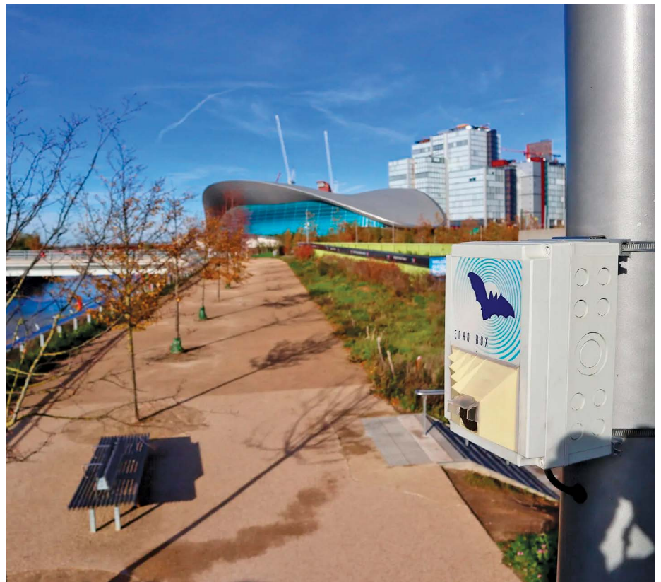
A smart monitor in London's Queen Elizabeth Olympic Park records bat activity.
