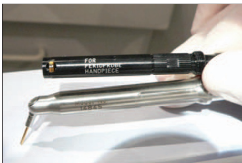
Fig. 3 Focused waveguide tip for use with CO 2 laser wavelength
