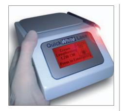
With a wavelength of  $810 \pm 5$  nanometers and 0.1-3 watts of power, you can choose from either continuous wave or pulsed depending upon your chosen application. These include soft tissue management, gingival incisions and excisions, second stage recovery of implants and vestibuloplasty.
