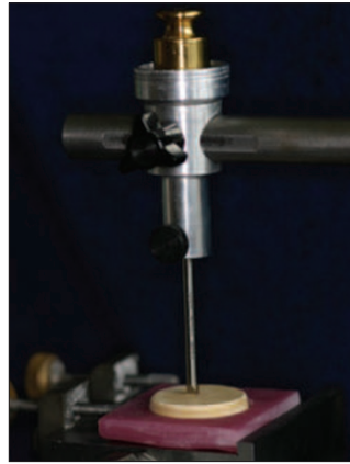
Photograph of abrasion device with 50 g weight applied
