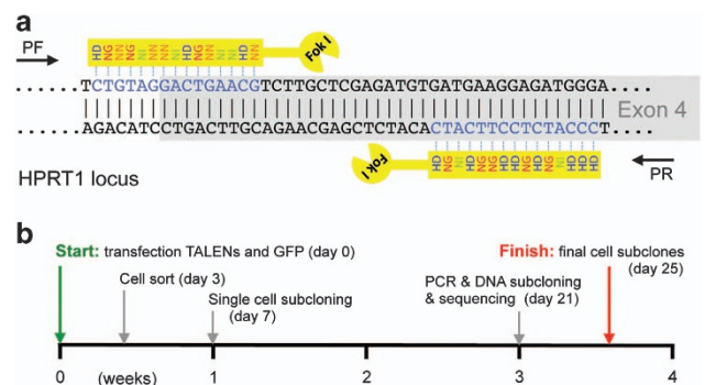
Figure 2. TALEN structure and timeline for TALEN-mediated modification. (a) Sequence representation of TALEN-mediated HPRT1 gene targeting. PF and PR are PCR primers. (b) Timeline of the entire procedure shows its unmatched efficiency.
