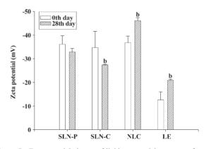
Figure 5. Zeta potential change of lipid nanoparticle systems after 28 d of storage at 37 °C. Each value represents the mean±SD. n=4. <sup>b</sup>P<0.05 significantly different compared to the data at d 0.
