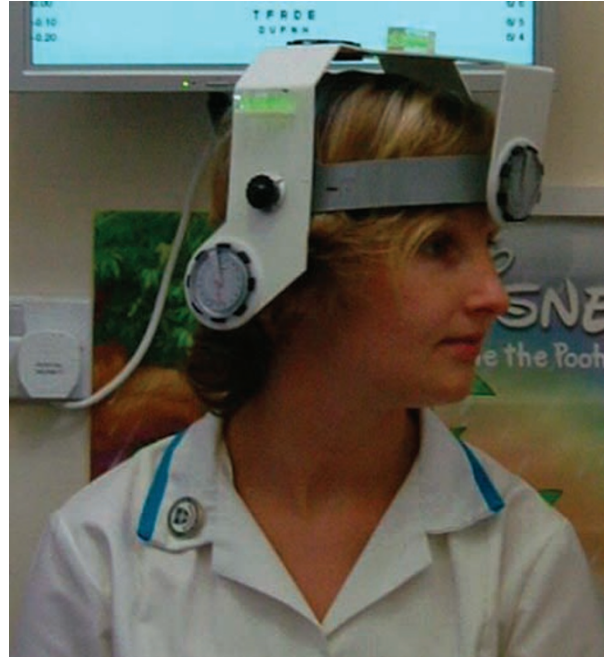
Figure 3 Inclinometer is displayed. This is a lightweight plastic device that fits securely on the patient's head and is simple to use. The head position or amount of motion can be read off the dials as shown.
