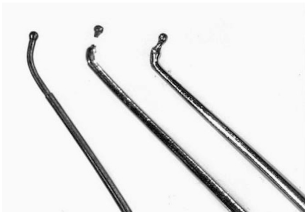
Figure 1 Lens manipulating instruments, the right extreme instrument with blunt bulged tip and narrow neck, the middle instrument with broken head from our case, compared with, left extreme, another instrument with no narrow weak point.
