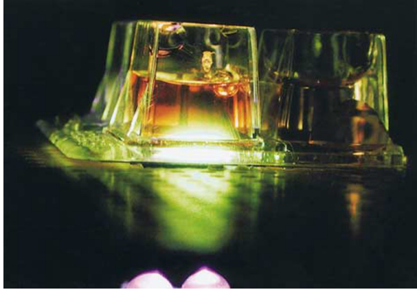
Figure 1 Irradiation procedure with double UVA-diode under the wells of the culture plate.
