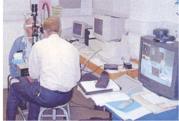
Figure 1 Live real-time video images are transferred along three ISDN lines. The remote examiner (screen) is able to switch between preset views to communicate with the SL operative and/or patient and family or to view images captured with the SL video camera.
