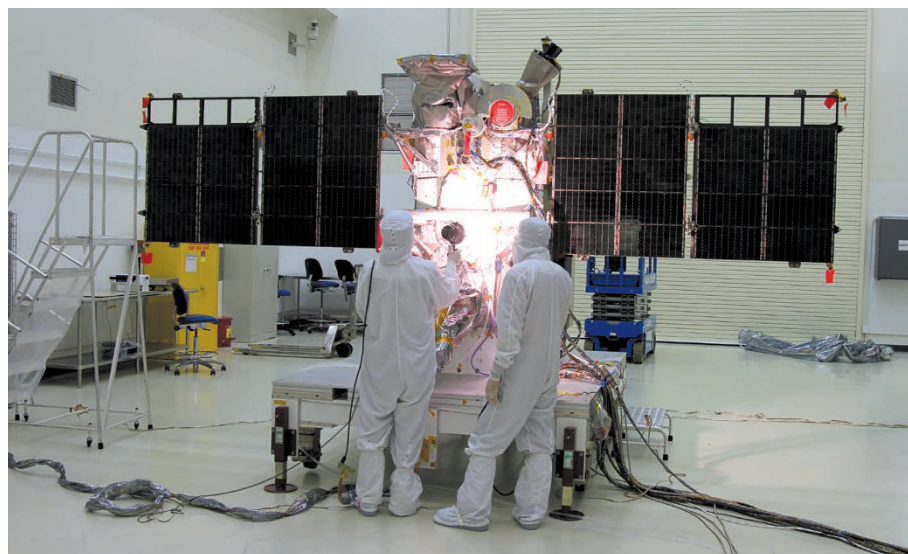
Workers test solar arrays on the DSCOVR satellite, which is now used to monitor space weather.
