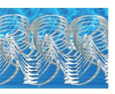
When the substrate returned to its original shape, the silicon buckled to form a range of structures less than a millimetre wide (pictured), including helices, boxes and flowers. These could then be assembled into larger configurations.
