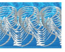
When the substrate returned to its original shape, the silicon buckled to form a range of structures less than a millimetre wide (**pictured**), including helices, boxes and flowers. These could then be assembled into larger configurations.
