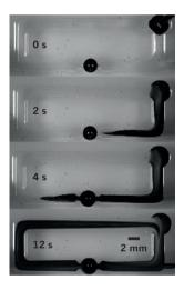
gallate anions diffusing to the droplet's surface. When a low-power electric field is applied, the rearrangement of charges at the droplet's surface causes it to shift in its constrained space in such a way that the surrounding solution flows past it (pictured).
